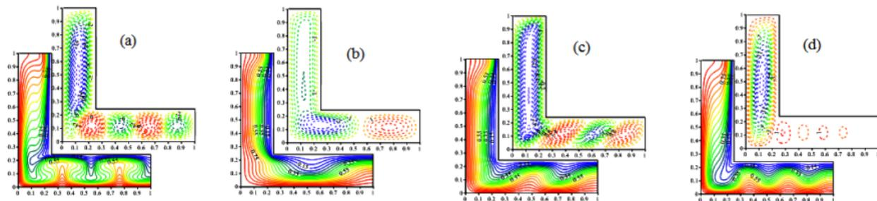
Figure 4: Streamlines (dash lines) and isotherms (solid lines) contours for (a)  $Ha = 0$ , (b)  $Ha = 100$  and  $\gamma = 0$ , (c)  $Ha = 100$  and  $\gamma = 30^\circ$  and (d)  $Ha = 100$  and  $\gamma = 90^\circ$
