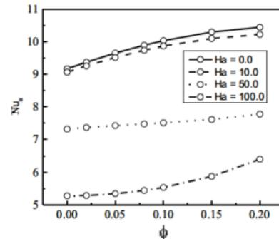
The average Nusselt number for different values of volume fraction  $\phi$  with different values of  $Ha$  at  $Ra = 10^6$ ,  $\theta = \frac{\pi}{2}$ ,  $\gamma = \frac{\pi}{4}$  and  $AR = 0.25$ .
