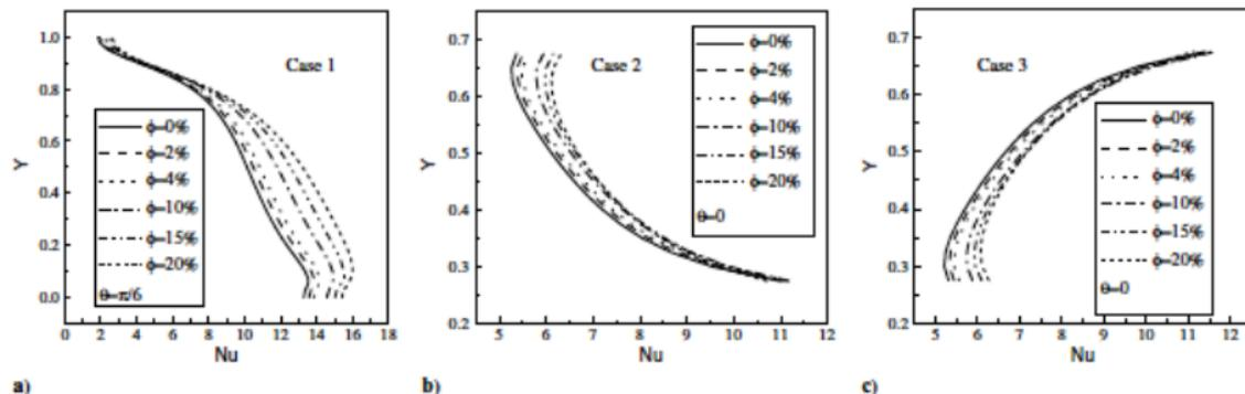
Fig. 16 Profiles of the local Nusselt number for  $\phi$  at  $b_L = 0.5$ ,  $B_L = 0.4$ ,  $b_R = 0.5$ ,  $B_R = 0.6$ , and  $Ra = 10^5$ .
