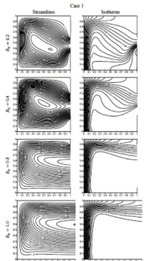
Fig. 7 Streamline and isotherm contours for different values of the open part length at  $b_1 = 0.5$ ,  $Re = 10^4$ ,  $\theta = \frac{\pi}{2}$  and  $\phi = 5\%$ .
