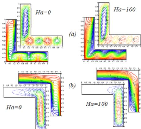
Figure 5: Streamlines (dash lines) and isotherms (solid lines) contours  $\vartheta = 0, 180^\circ$
