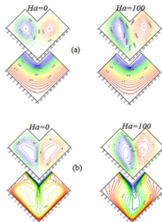
Figure 6: Streamlines (dash lines) and isotherms (solid lines) contours  $Ra = 10^3, 10^6$
