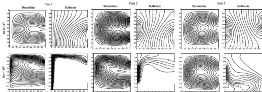
Fig. 11 Streamline and isotherm contours for different values of  $Ra$  at  $b_2 = 0.5$ ,  $B_1 = 0.6$ ,  $\theta = \xi$  and  $\phi = 5\%$ .
