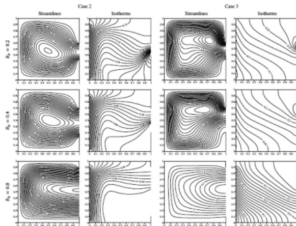
Fig. 8 Streamline and isotherm contours for different values of the open part length at  $b_1 = 0.5$ ,  $\theta_1 = 0.1$ ,  $b_2 = 0.5$ ,  $Re = 10^4$ ,  $\theta = \frac{\pi}{2}$  and  $\phi = 5\%$ .
